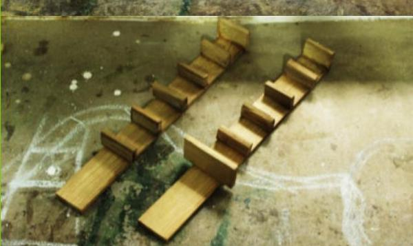
Fixture for holding & maintaining the uniform gap between the members
