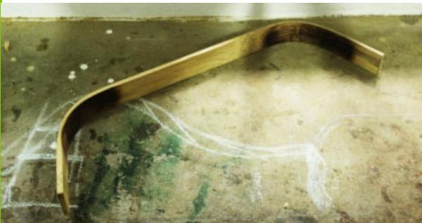
The bent profile member of the stool. The bamboo is bent using Hot Blower Gun.
