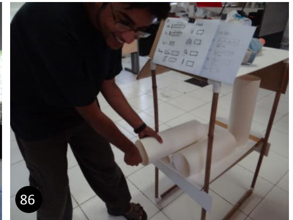
Fig 83 - testing one of the interface layouts Fig 84 - accessibility from the front side - monitor interface may have an affordance of hand rest Fig 85-86 - testing the oxygen cylinder orientations- horizontal/vertical to understand ease of access, replacing and setting up connection.
