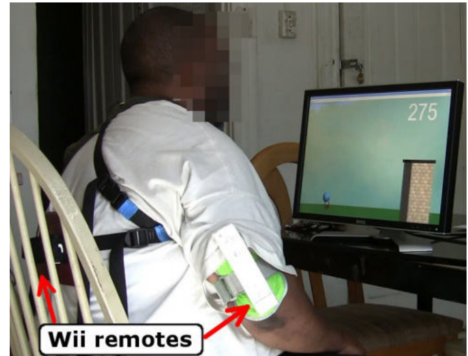
Figure 3.9 - Participant playing the game with multiple Wii remotes strapped to arm and back to detect compensatory motion.
