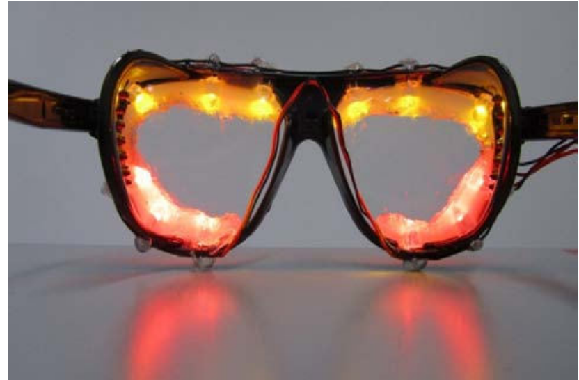
Figure 7: Alerting system with LEDs (IAD: Ringwald u.a., 2011)
