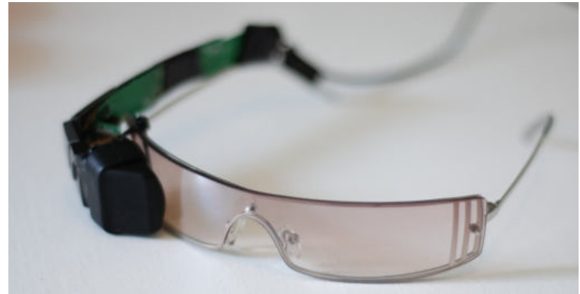
Figure 8: Concept for a head mounted visual system on the side of the visual range (Kellersmann 2011)
