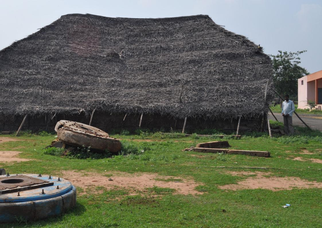
If we see closely, the wheels which were discarded are also made from wood. They used a technique to make a wheel out of logs of wood. They made cubiods out of the logs and then stacked one over another to make a disc with some thickness. Over this disc, planks of wood are used to revert it permanently in place. The axel was also used to made of wood. For this year, Bharat Heavy Electricals Limited (BHEL) supplied steel wheels and axles as shown in the pics.
