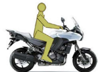
2013 Kawasaki Versys 1000 Calculated seat height: 33.5" Forward lean: 5° Knee angle: 95° (smaller number means more bent) Hip angle: 99° (smaller number means more crouched)
