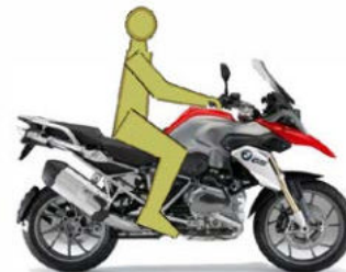
2013 BMW R1200GS Calculated seat height: 34.4" Forward lean: 6° Knee angle: 96° (smaller number means more bent) Hip angle: 99° (smaller number means more crouched)
