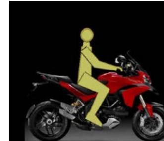
2013 Ducati Multistrada 1200 Calculated seat height: 33.0" Forward lean: 3° Knee angle: 91° (smaller number means more bent) Hip angle: 99° (smaller number means more crouched)
