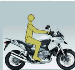
2012 Honda Crossrunner VFR1200X Calculated seat height: 33.8" Forward lean: 6° Knee angle: 93° (smaller number means more bent) Hip angle: 98° (smaller number means more crouched)
