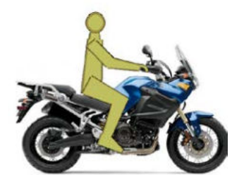
2012 Yamaha Super Tenere XT1200Z Calculated seat height: 33.1" Forward lean: 3° Knee angle: 94° (smaller number means more bent) Hip angle: 96° (smaller number means more crouched)
