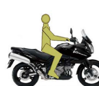
2010 Suzuki V-Strom 1000/DL1000 Calculated seat height: 33.7" Forward lean: 0° Knee angle: 90° (smaller number means more bent) Hip angle: 103° (smaller number means more crouched)
