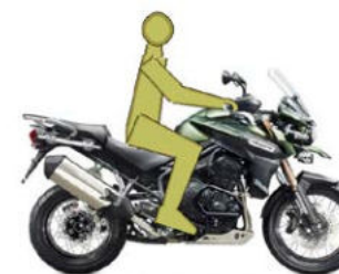
2014 Triumph Tiger Explorer XC Calculated seat height: 33.8" Forward lean: 3° Knee angle: 92° (smaller number means more bent)
