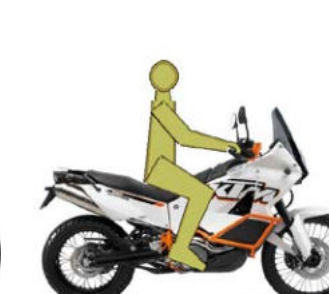
2012 KTM 990 Adventure Calculated seat height: 34.3" Forward lean: 2° Knee angle: 90° (smaller number means more bent) Hip angle: 99° (smaller number means more crouched)
