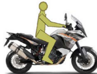
2013 KTM 1190 Adventure Calculated seat height: 34.0" Forward lean: 6° Knee angle: 95° (smaller number means more bent) Hip angle: 99° (smaller number means more crouched)
