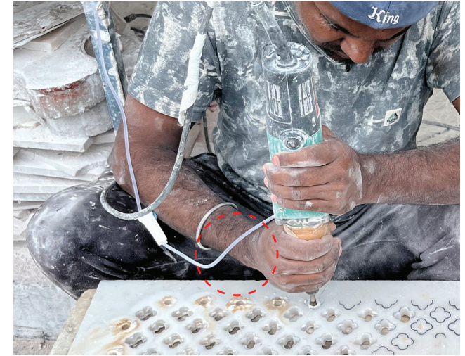
Fig 20.7.3: Issue of Pipe Falling On Hand
