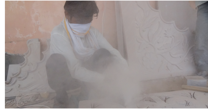
Fig 12.1: Dust Emission While Stone Cutting
