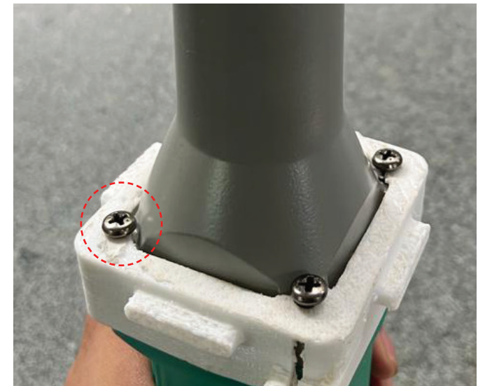
Fig 23.2.3: User Test For Clamping By Existing Screws
