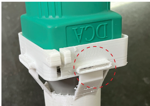
Fig 20.2.4: Extrusion to Channel The Air Outwards
