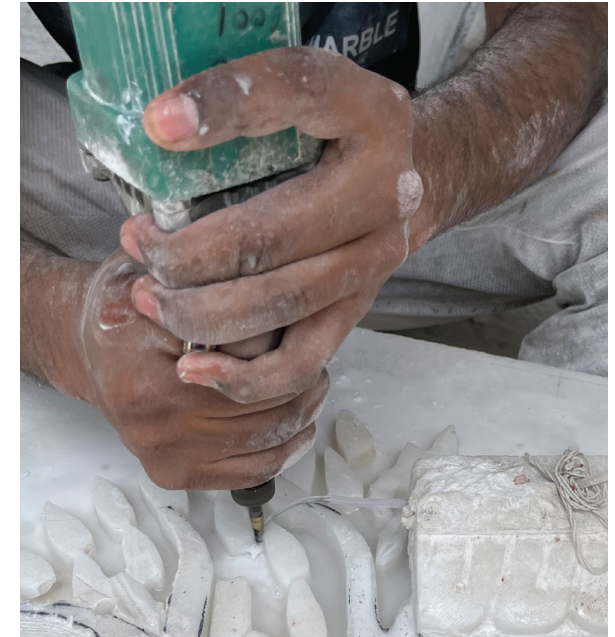
Fig 15.5.3: Dust Emission With Water Supply
