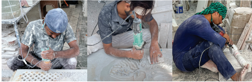
Fig 20.3.1: Working Hand Supported on Table/Body
