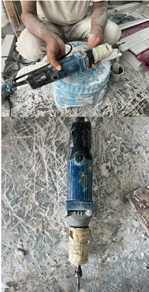
Fig 15.7.1: Grip Customization With Tapes
