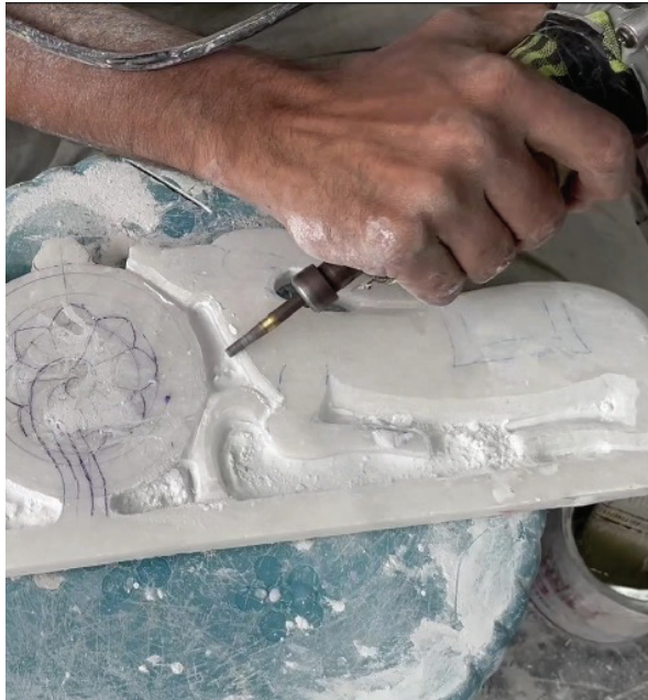
Fig 15.5.1: Dust Emission When Machine Angled
