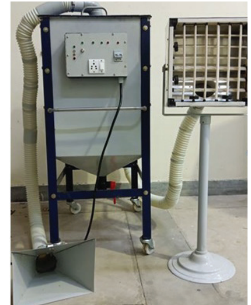
Fig 12.4: Dust Suction Machine
