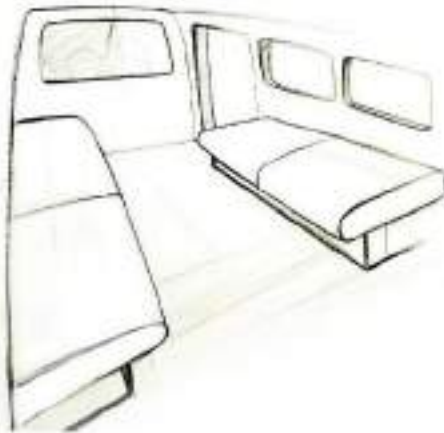
Two Parallel Seating, more passenger capacity, but ingress/egress is a pain, due to the narrow door.
