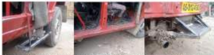
Rear Footboard is standard. Irregular pattern on the Side foot-board
