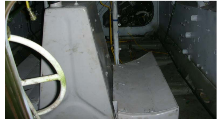
No Harness & Cushioning on the Seats
