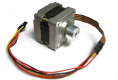
12V, 160mA 5 wires, unipolar stepper* motor 1.8 degree step angle
