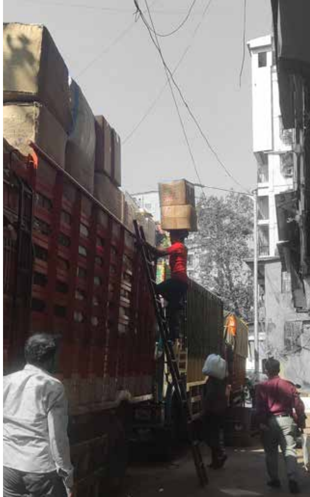
Higher level of cargo bed - Difficulty for loading and Unloading as well as Unsafe for pedestrians and workers.
