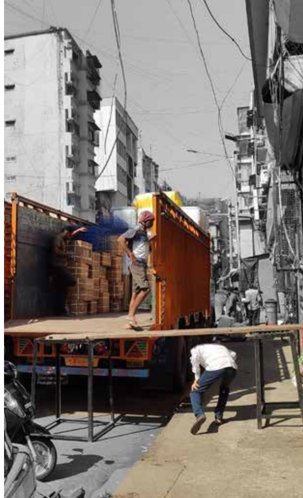
Higher level of cargo bed - Difficulty for loading and Unloading as well as Unsafe for pedestrians and workers.
