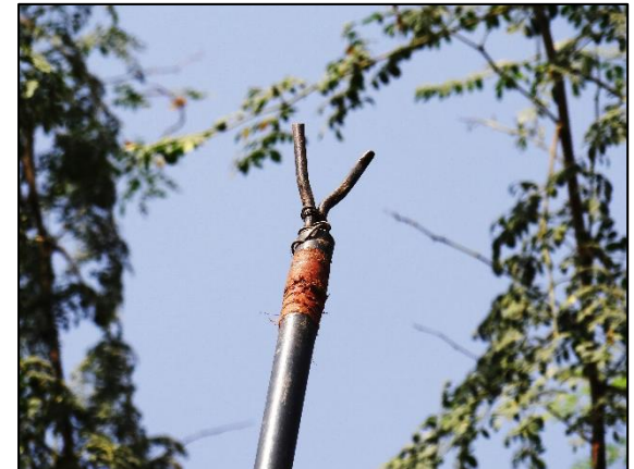
Fig.8: Tool made-up of a PVC pipe and steel rod
