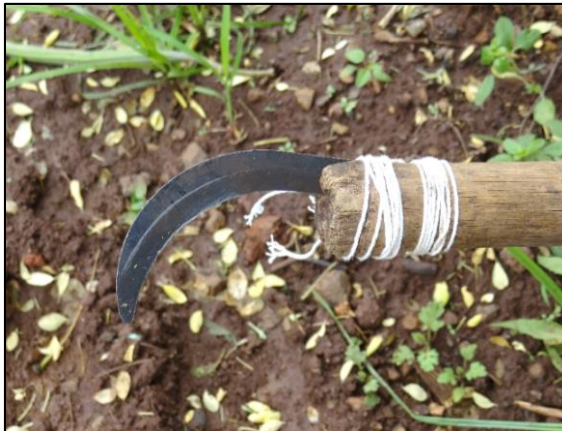
Fig.6: Tool made-up of a bamboo and small Khurpe
