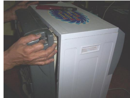
Fixing of the rear panel-no tool required
