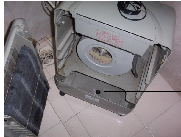
Drain cock is to be removed from inside the tank
