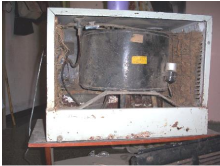
Steel body rusts badly due to water
