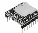
dfplayer mini mp3 module (for storing bird voice audio file)
