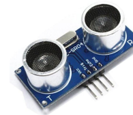
HC-SR-04 Ultrasonic Distance Sensor (for detecting distance)
