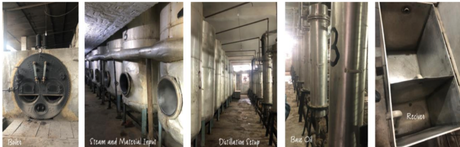
Figure 16 Equipment for steam distillation , Source: Author
