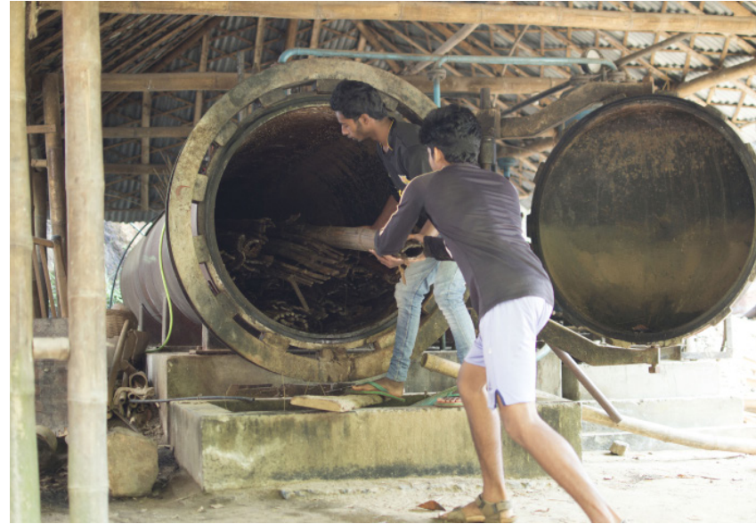
Fig 32 - Gas pressure impregnation(top)
