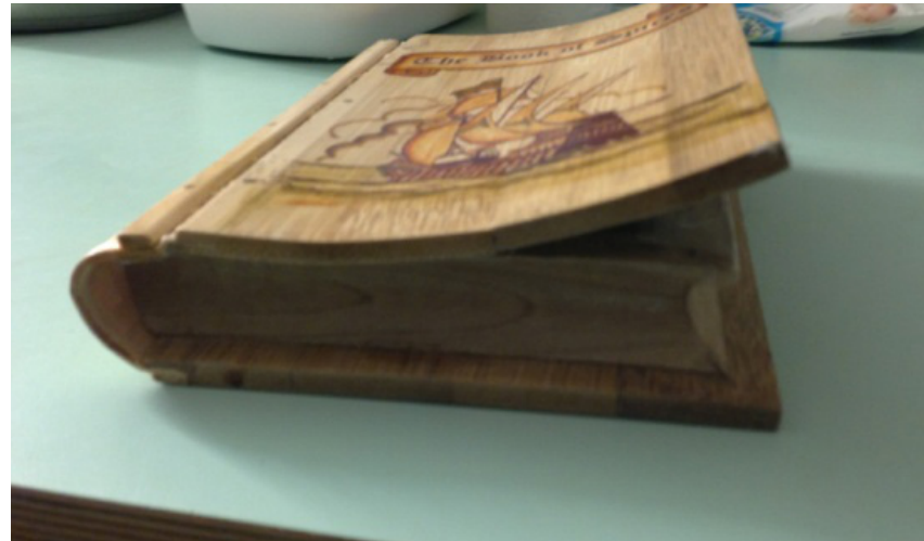
Fig 39 - Warping issue at extreme temperatures
