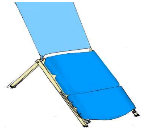
Mechanism for making it compact #1; Sliding Leg rest
