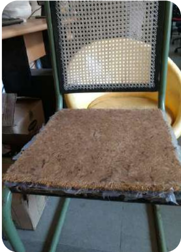
Prefabricated coir silicon sheet bolted on the seat of an office chair.
