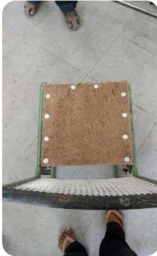
Prefabricated coir silicon sheet bolted on the seat of an office chair.
