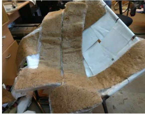
Top from left; Coir silicone sheet fabrication by sandwiching felt between silicone layers, Fabrication of steel chassis
