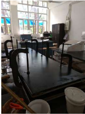
Top from left; Coir silicone sheet fabrication by sandwiching felt between silicone layers, Fabrication of steel chassis
