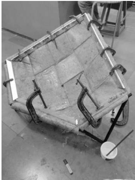
Top from left; Coir silicone sheet fabrication by sandwiching felt between silicone layers, Fabrication of steel chassis
