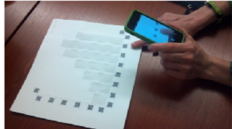
Figure 1. The Tactile Graphics with a Voice system in use. The subject is using the finger pointing mode to select which QR code to scan.
