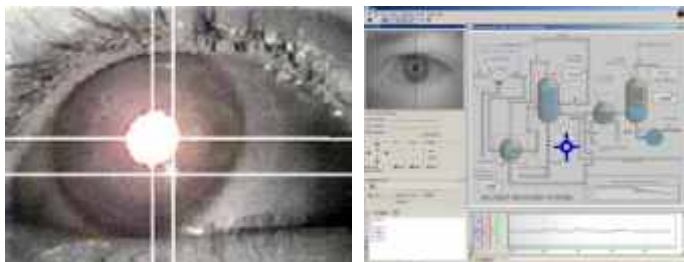
Figure 2: The large white circle is actually the dark pupil and the small circle at the lower left of the pupil is the bright corneal reflexion.
