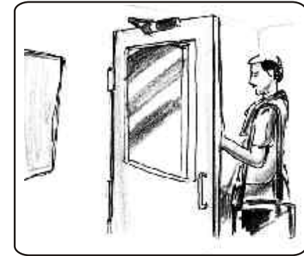
AC compartment door shuts immediately because of hydraulic hinge
