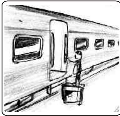
Steps to board the train are vertical and height of platform varies
