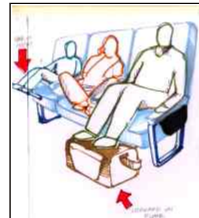
Users respond differently with interesting postures for sitting. Middle passenger has problems in movement.
