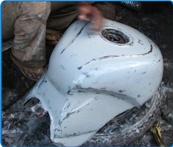
Sheet metal tank being worked for painting
