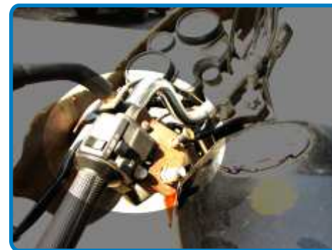
Switches for Emergency light and Siren
