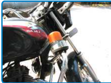
Emergency signal lights
