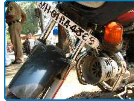
Emergency signal light and Siren
