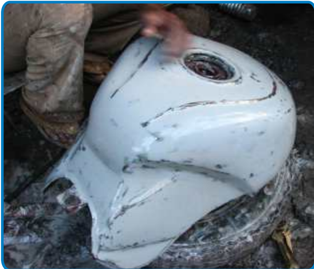
Sheet metal tank being worked for painting
