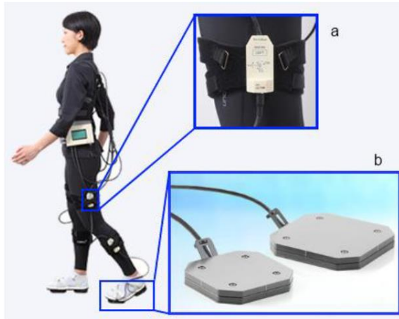
Figure 7: WS system based on (a) inertial sensors; and (b) wearable force plates [23].
