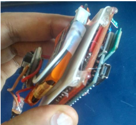
Figure 14: Combined height of shank sensor and power module. The LiPo battery was glued underneath the motion sensor module, separated by a layer of 0.5mm styrene for protection and prevent possible short circuit or thermal damage.
