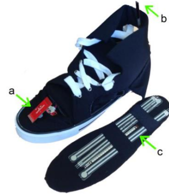
Figure 4: Instrumented shoe from Smartxa Project: (a) inertial measurement unit; (b) flexible goniometer; and (c) pressure sensors which are situated inside the insole [23].
