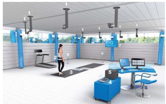
Figure 6: Example of NWS system: BTS GaitLab configuration. (1) Infrared video cameras; (2) inertial sensor; (3) GRF measurement walkway; (4) wireless EMG; (5) workstation; (6) video recording system; (7) TV screen; (8) control station [23].
