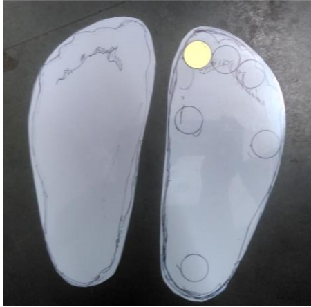
Figure 9: Cutout of the styrene sheet for left and right foot. The shiny circular coin was the piezoelectric sensor, placed on one of the circular markings of the pressure points of the foot.
