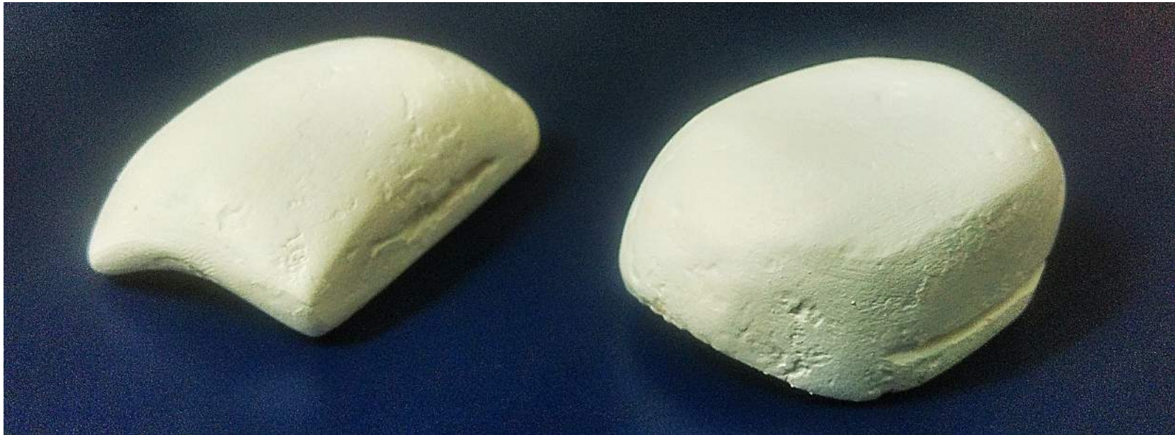
Figure 30: Two product form explorations for the ankle of the foot. The side groove is slot for passing velcro.
