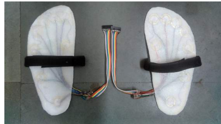
Figure 14: Image shows the finished prototype of the foot sensor module. Black was the Velcro and the white sheet was the sponge layer glued on top of the styrene sheet and piezoelectric sensors.
