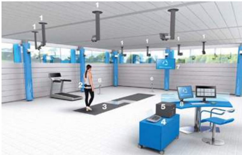
Figure 6: Example of NWS system: BTS GaitLab configuration. (1) Infrared video cameras; (2) inertial sensor; (3) GRF measurement walkway; (4) wireless EMG; (5) workstation; (6) video recording system; (7) TV screen; (8) control station [5].
