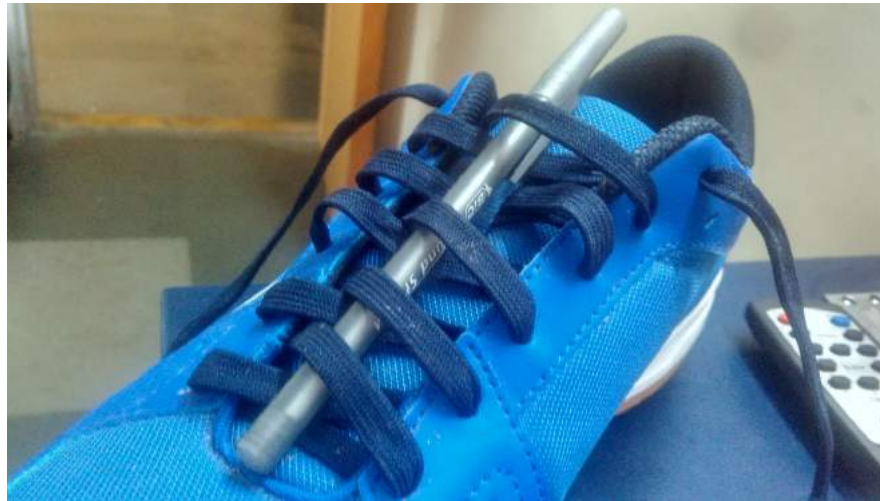
Figure 26: Image shows how the single rod—shown here by a pen—style locking mechanism fits through the lace of the shoe. Stability is the main problem faced by this style of locking of the product to the shoe.
