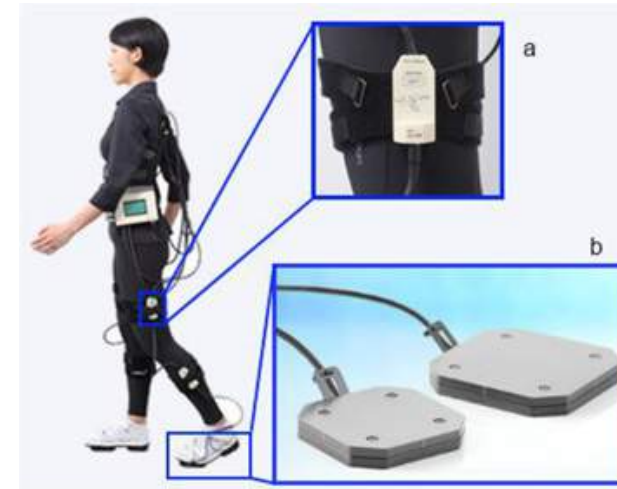
Figure 7: WS system based on (a) inertial sensors; and (b) wearable force plates [5].
