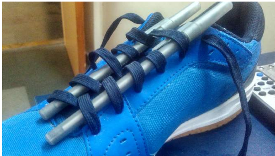
Figure 27: Image shows how the double rod—shown here by two pens—style locking mechanism fits through the lace of the shoe. This type of locking to the shoe is more stable as compared to single rod styled product locking to the shoe.
