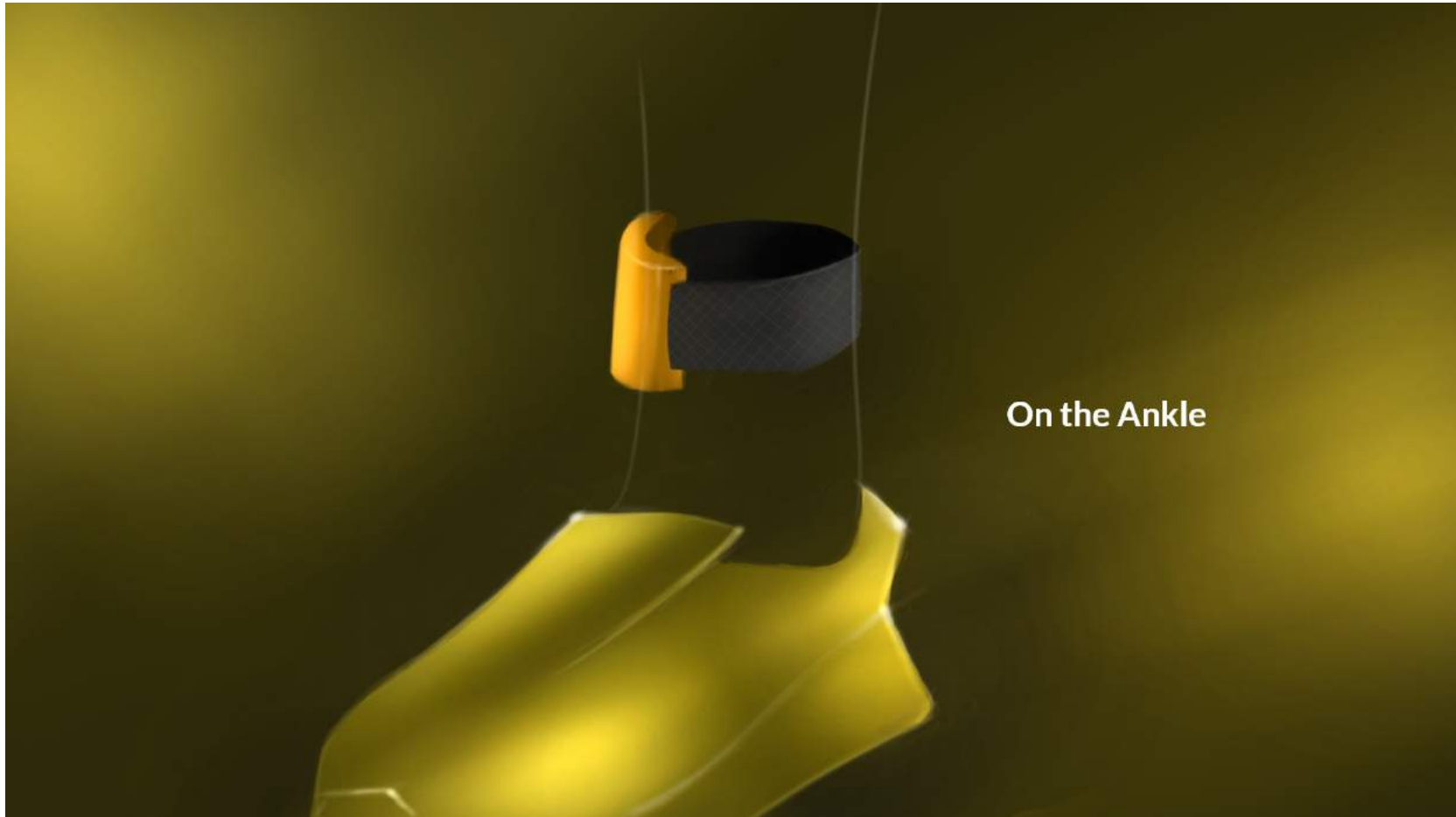
Figure 21: Non-photorealistic rendering of the product(orange colored) tied on the ankle of the foot, using velcro(textured grey colored).
