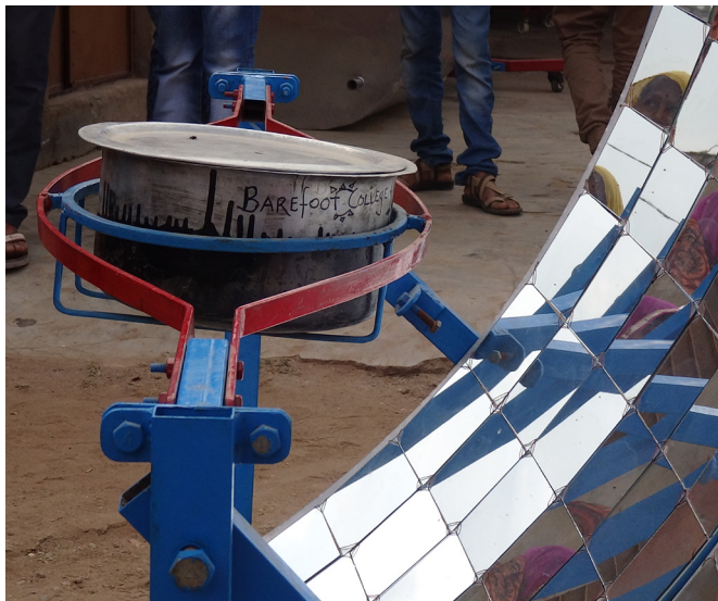
Fig 19 - Solar cooker made by solar mamas in Barefoot college.
