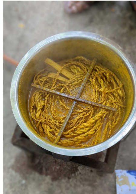
Boiling with Turmeric and little red for getting golden orange rope
