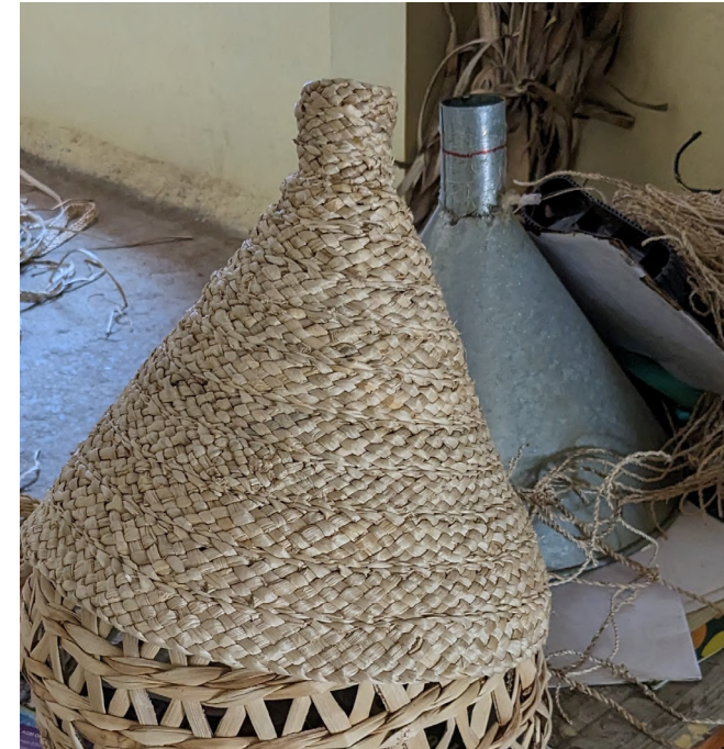
Braided sheaths of various widths are stiched over a mould
