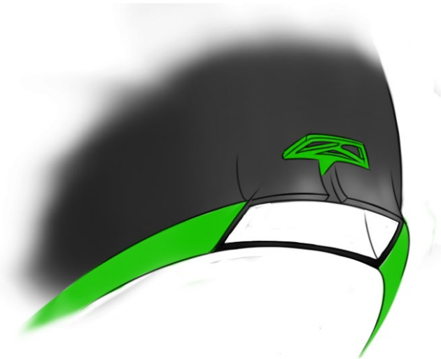
Fig.75: Suction mount cavity on helmet
