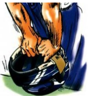
Fig.24: Fitting inner liner
