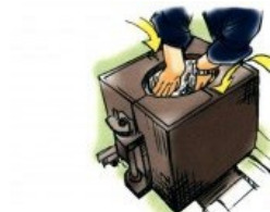
Fig.19: Moulding fibre layers
