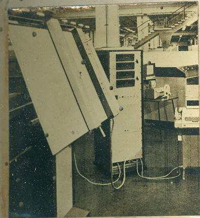
The automated computerized drafting machine has a precision table with a drawing area from 4' x 4' to 6' x 20', a travelling beam and carriage which moves the drawing device and servodrive motors to control the movement of the system. The drawing board holds one or several stylus which may be either a capillary pen or a metal scribe. Only one stylus is in operation at any given time.
