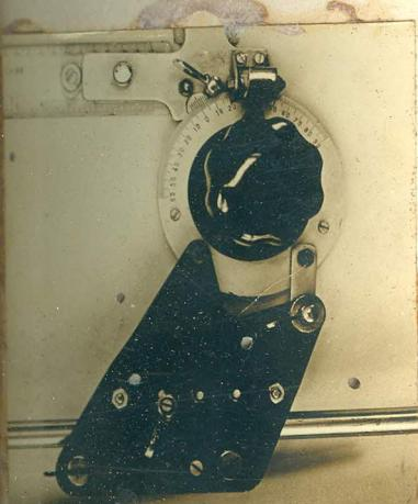
The upper plate has got graduation of zero degree to 60 degrees anticlockwise and zero degree to 90 degrees in clock wise direction having the zero line coinciding the 45 degree line between both the scales. This protractor has got a knob at the middle made of U.F.resin.
