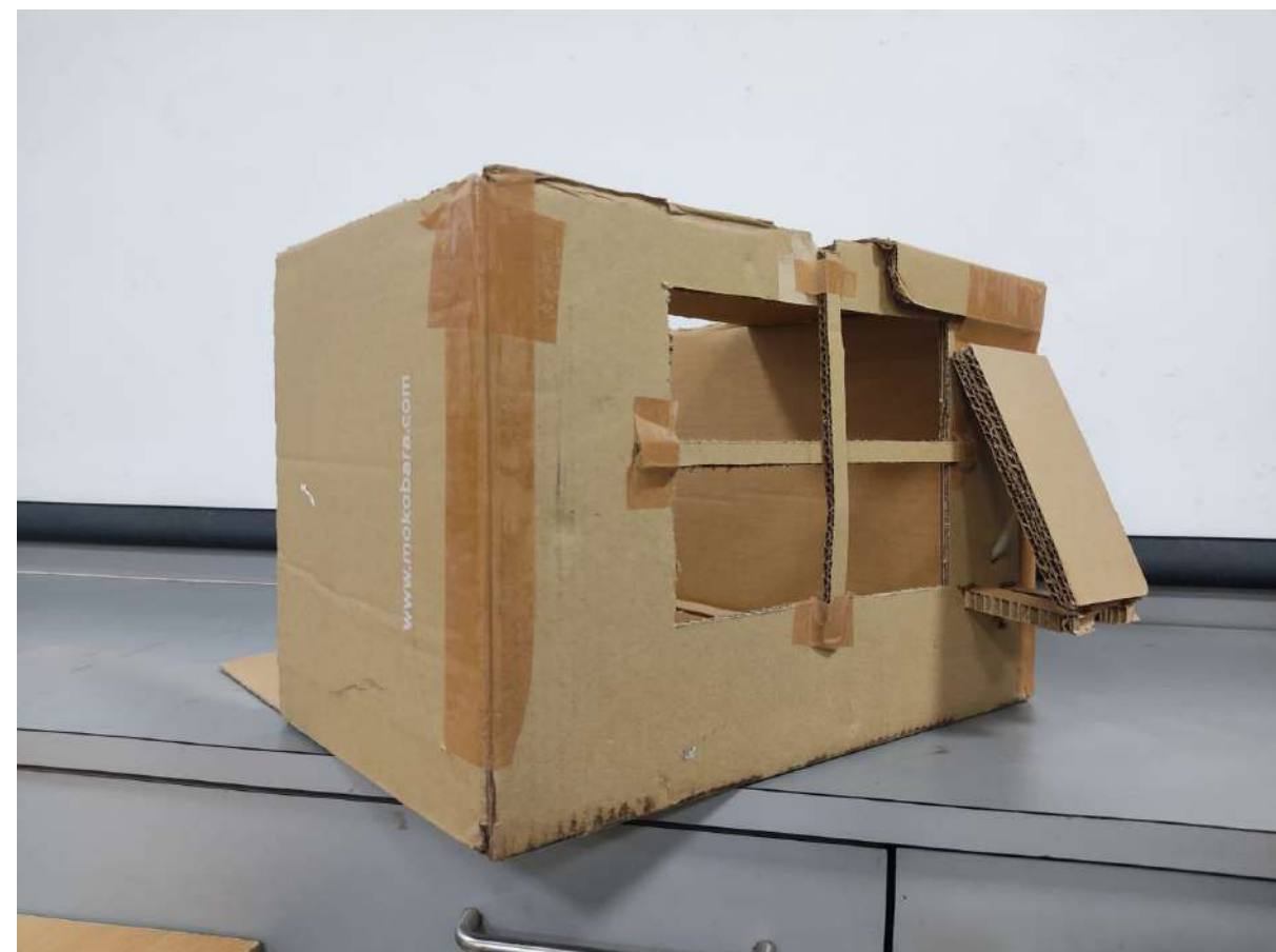
Mockup of the suggested changes by Prof. Rane sir. Major change was to install SAH near the window to reduce the pressure drop
