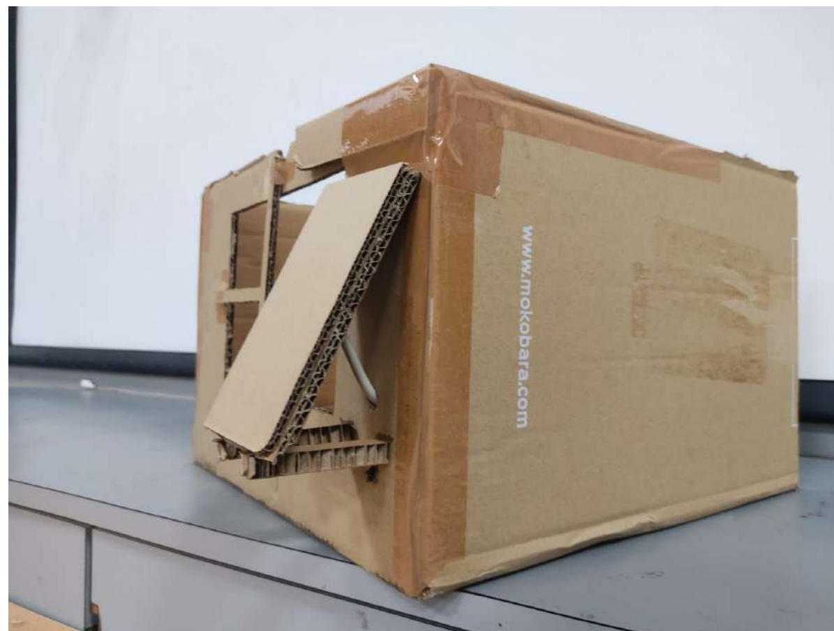
Mockup of the suggested changes by Prof. Rane sir. Major change was to install SAH near the window to reduce the pressure drop
