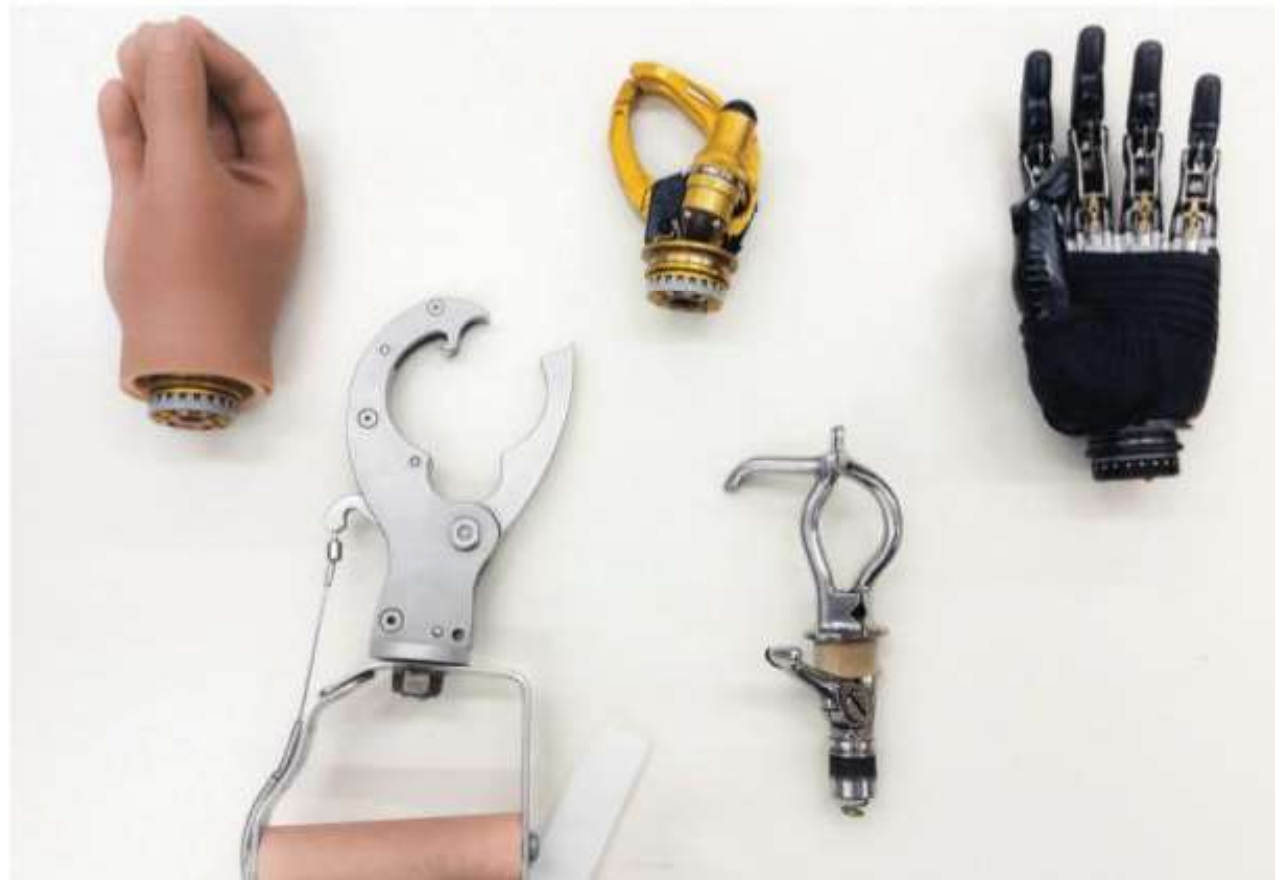
Figure 13: Examples of currently available prosthetic hands. Body-powered terminal devices and myoelectric hands interpret muscle signals from a patient's body to actuate battery-powered robotic motors.
