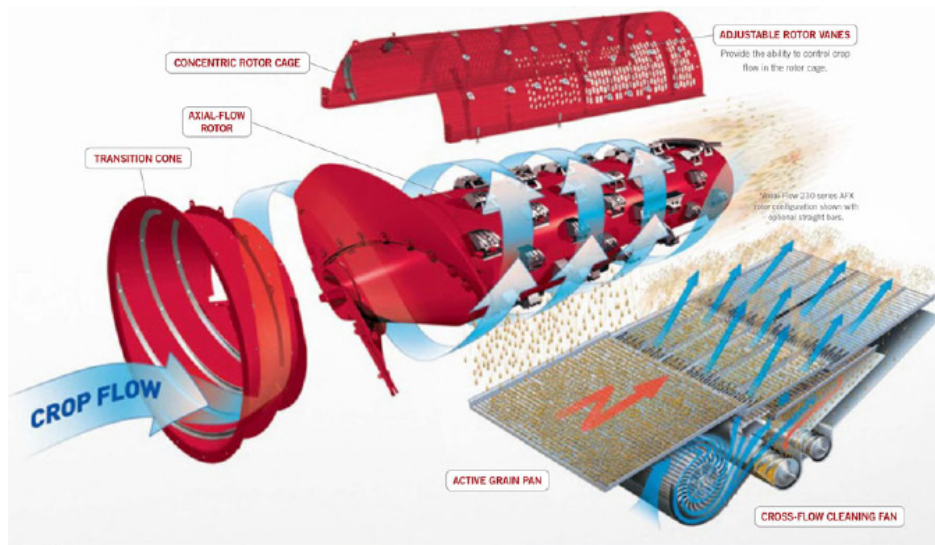
Figure 5-8. Schematic of axial flow threshing unit[16]
