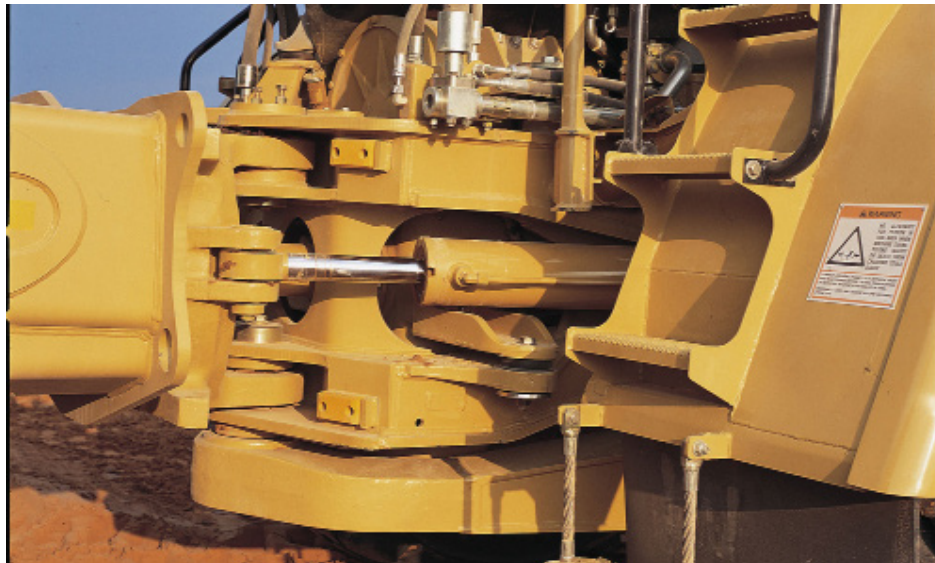
Figure 11-7: Articulated steering mechanism[24]
