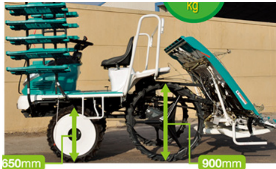
Figure 11-10 Existing wheel dimensions used in machines operating in mud[27]
