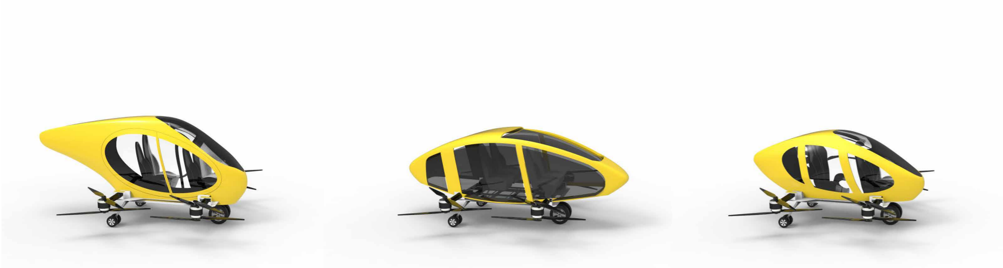
Image 36 : A single chassis can be used for various different form of the fuselage as per the requirement
