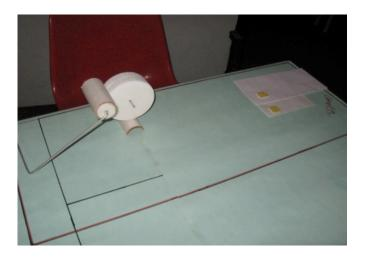
This is side wise feeding mechanism, in this case the hand movements are very less thus convenient for feeding letters and easy positioning.
