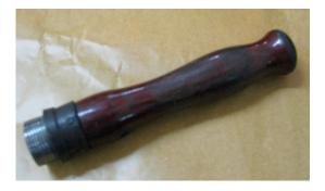
Metal with threads is fitted on wooden handle, casted block after inserting date is locked on the threads.
