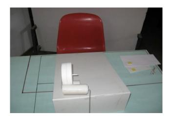
This is front feeding mechanism, position of rollers are in front of eyes at a particular height thus convenient for positioning letters properly.
