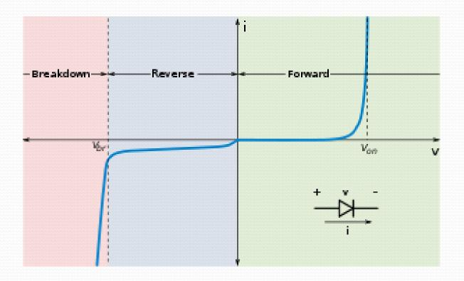
I-V diagram for a <u>diode</u> an LED will begin to emit light when the on-<u>voltage</u> is exceeded. Typical on voltages are 2-3 <u>Volt</u>
