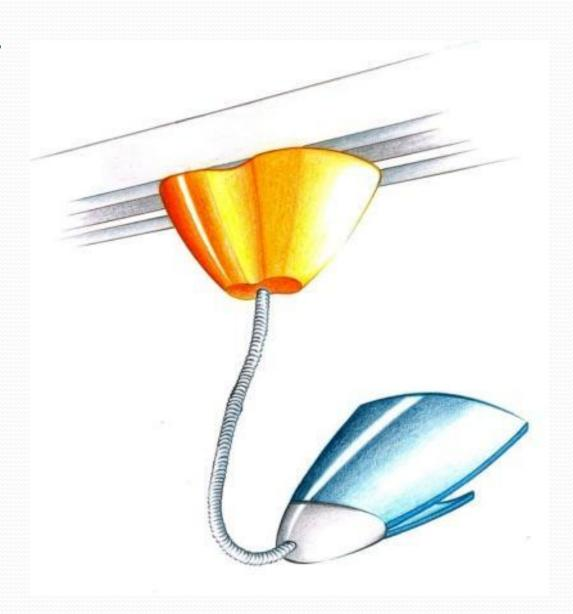
Formed acrylic sheets and RBG controlled led's, track light which can be fixed on a track on wall:
