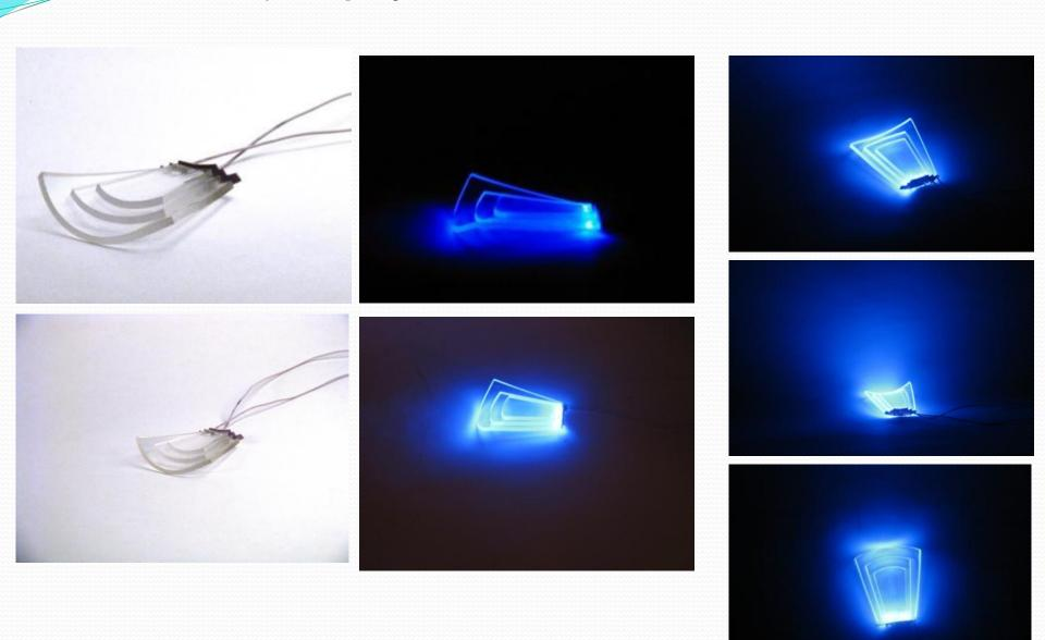
Acrylic bars fixed to circular base with led inserted in it:
