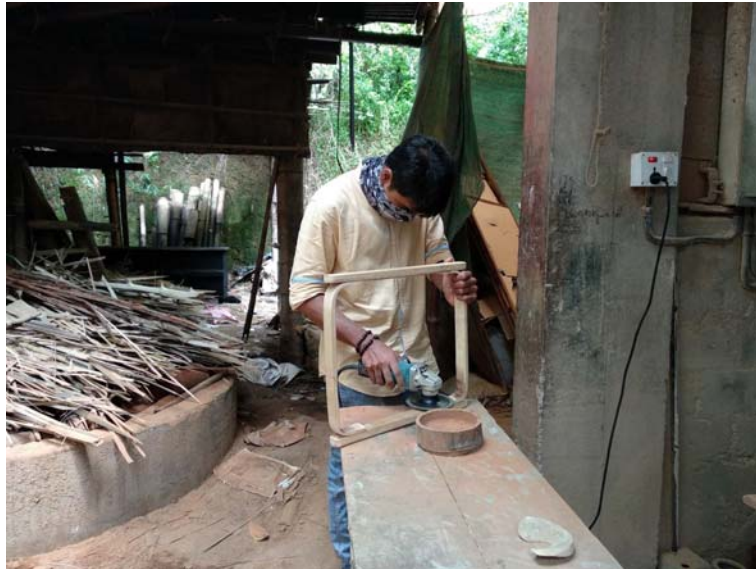
Finishing the frame using an angle grinder
