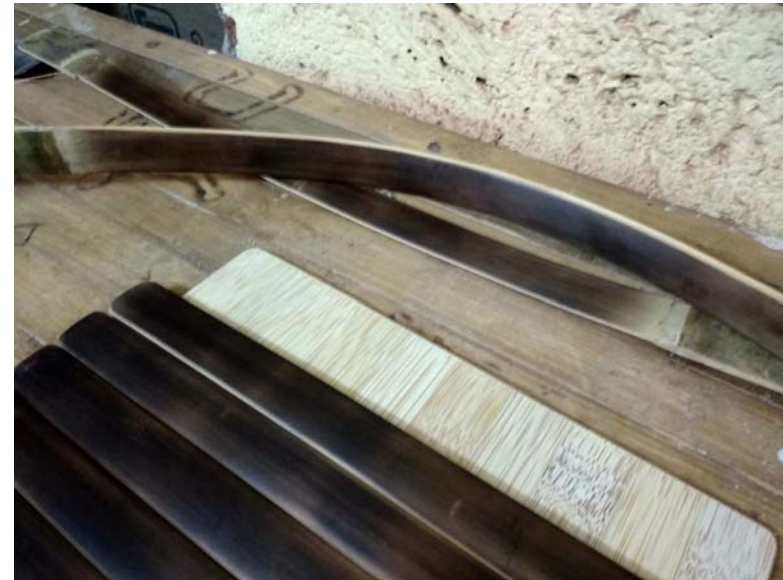
Charring the seat pieces and the backrest pieces using a blowtorch
