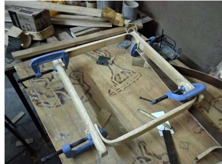
Assembling the seat frame
