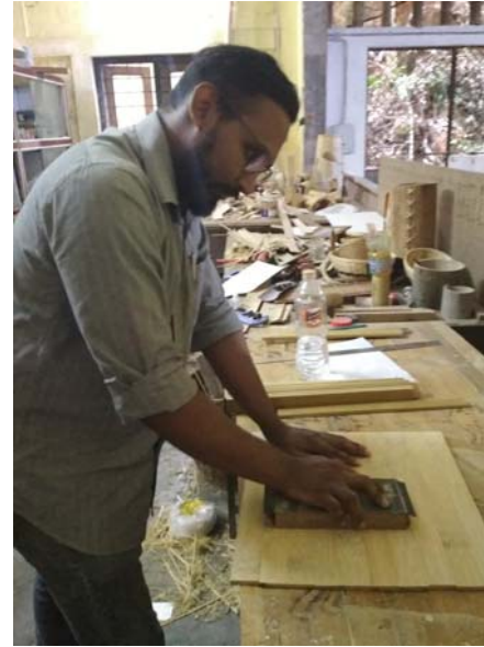
Finishing the seat piece using an angle grinder and then using sand paper
