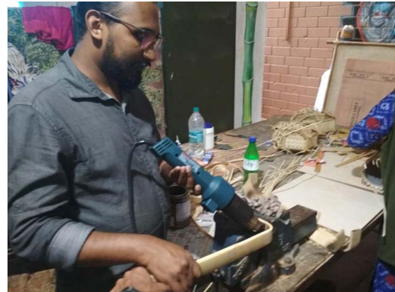
Bending the reapers using hot air gun
