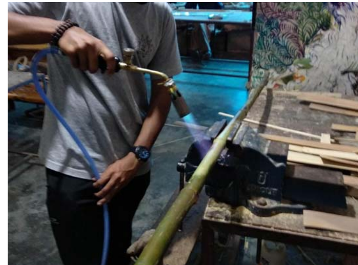
Straightening the strictus pieces using an LPG blow torch
