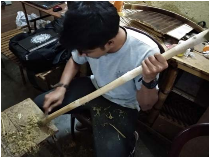
Scraping the surface of the bamboo using a knife
