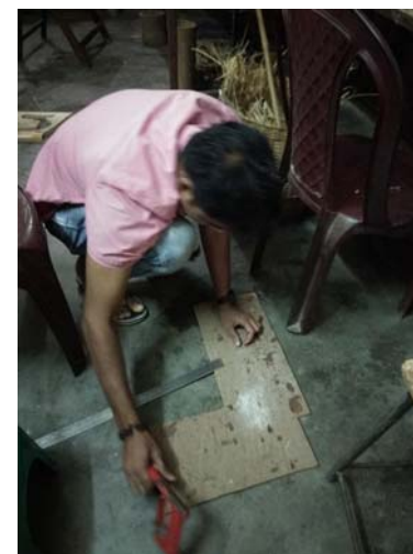
Scraping the surface of the gigantus bamboo reapers using a knife
