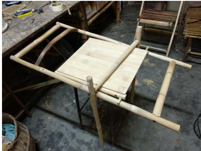
Final assembly of the seat and leg pieces
