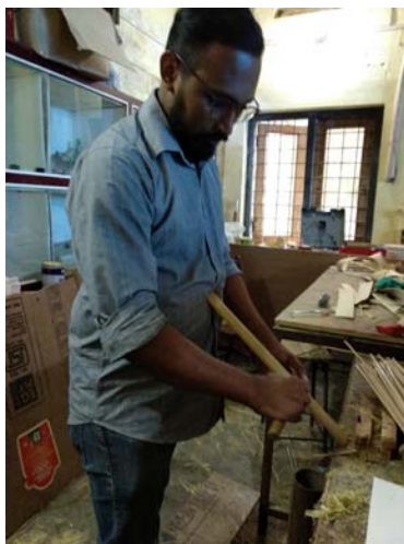
Scraping the surface of the gigantus bamboo reapers using a knife
