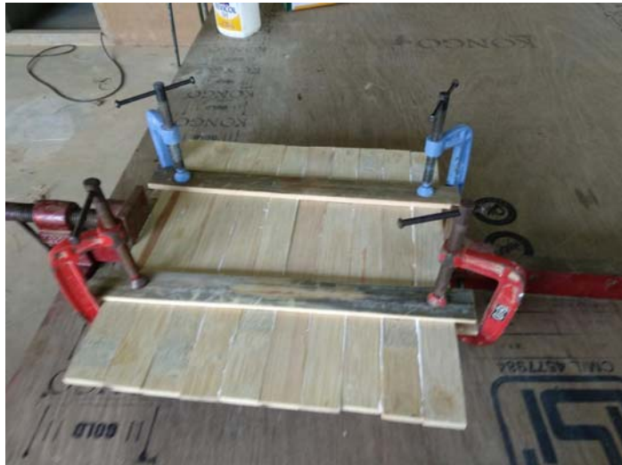
Sticking gigantus bamboo reapers to make the seat
