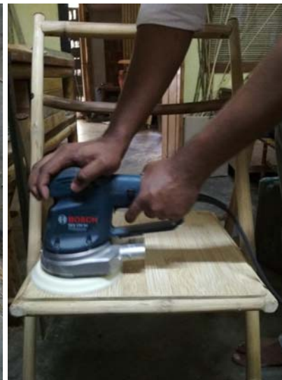
Final sanding and finishing
