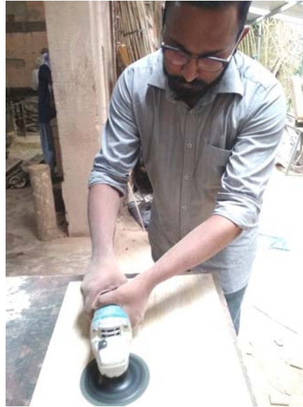
Finishing the seat piece using an angle grinder and then using sand paper
