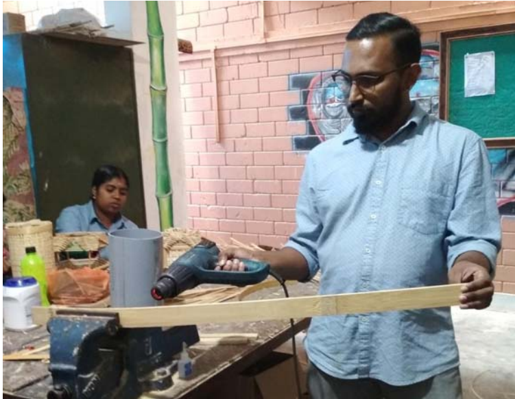
Bending the reapers using hot air gun
