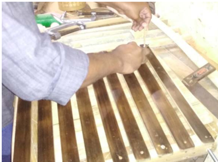
Nailing the seat panels to the frame
