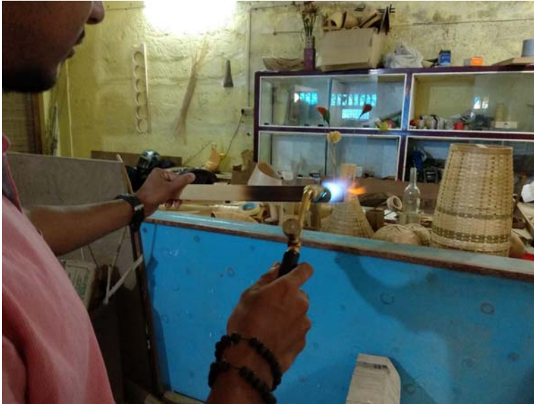
Charring the seat pieces and the backrest pieces using a blowtorch
