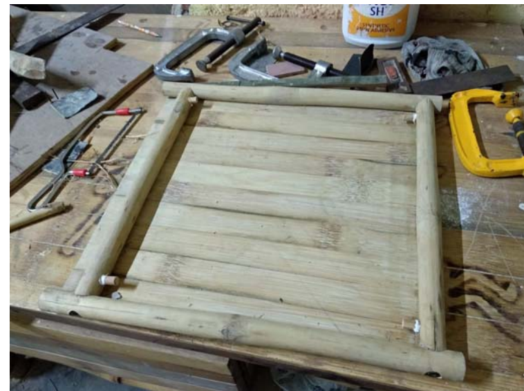
Assembling the seat piece to the strictus frame
