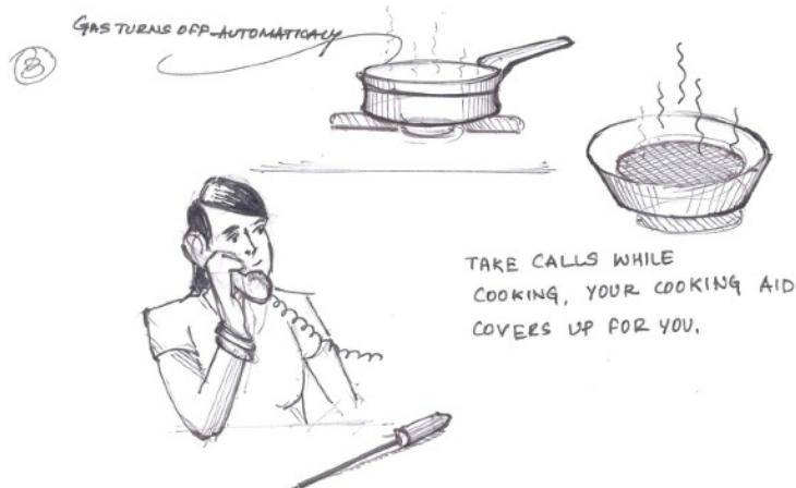
*The cooking aid will cover up for the users mistakes. In this case, the device will reduce heat accordingly so as to not burn the food.*
