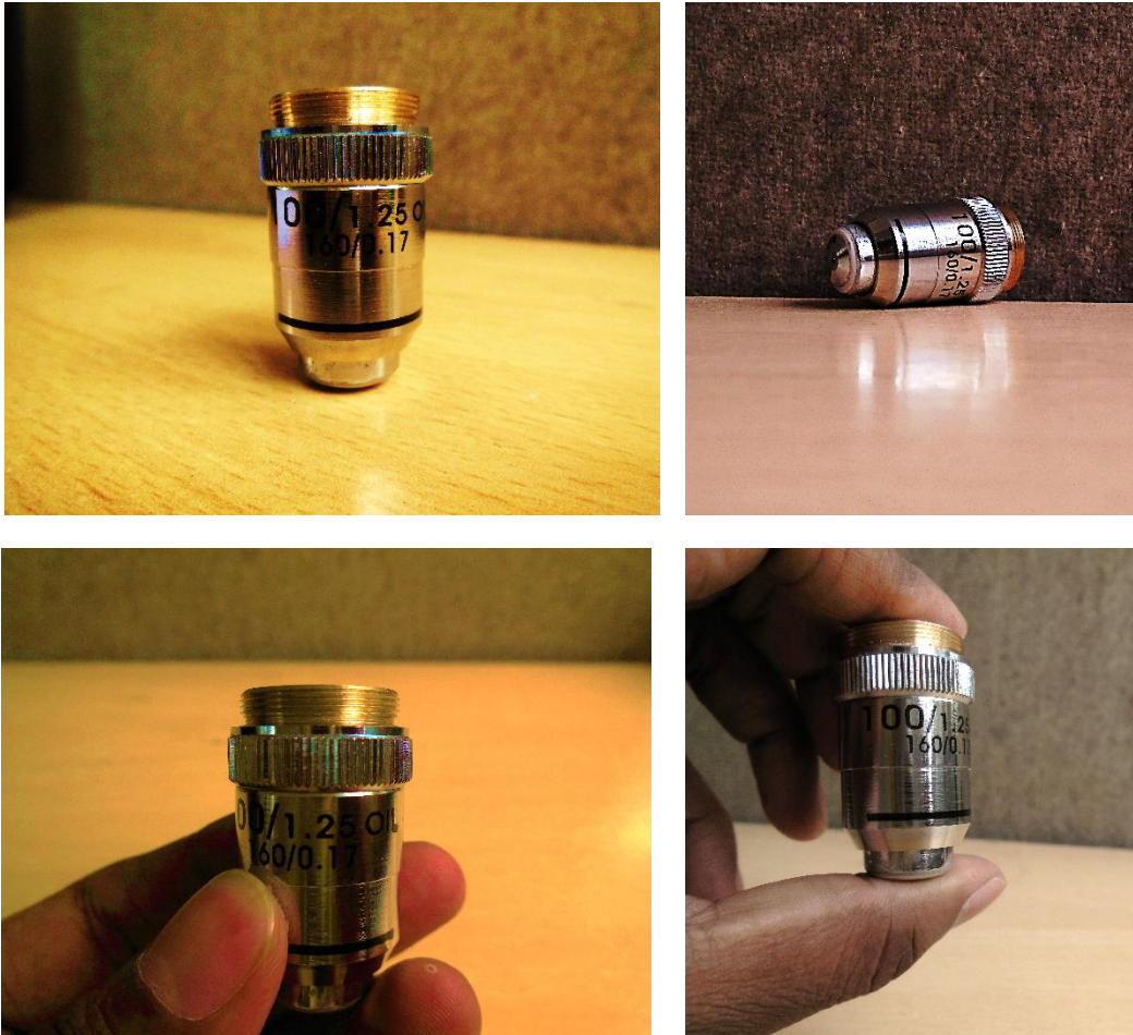
Image 56-59. Different views of Oil emersion lens
