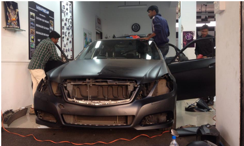
Image 5.1.1 Wrapping a vehicle in the Workshop In Pune
