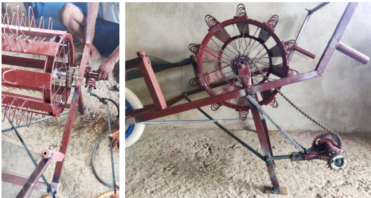
Figure 6.11: Modifications done to reinforce the chassis and improve power transfer
