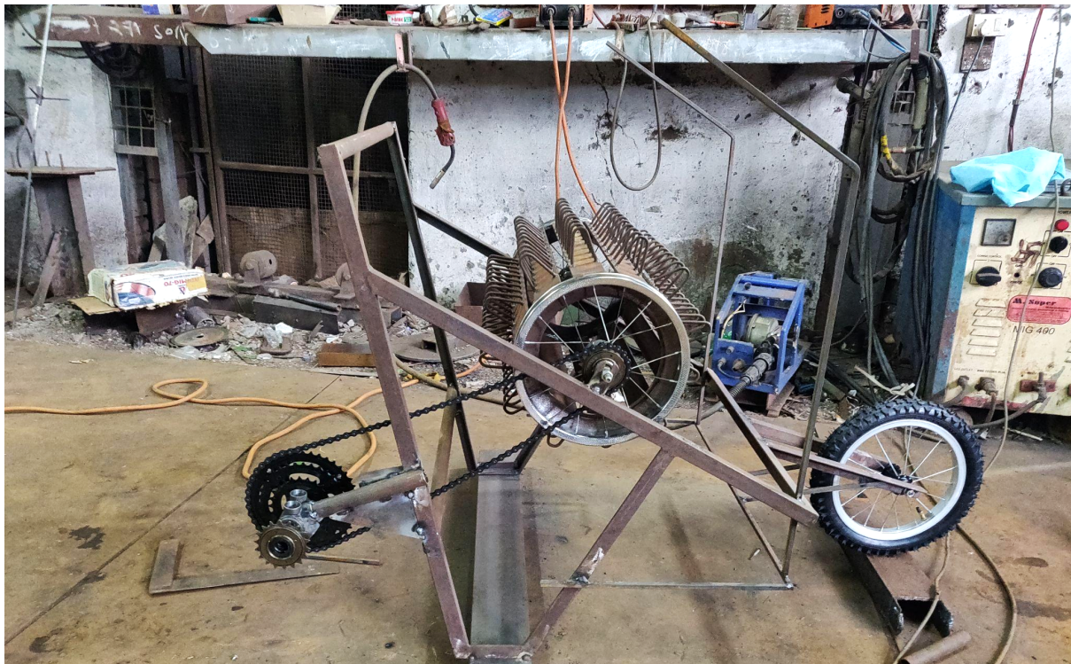
Figure 6.19: Fabrication of base thresher prototype 3.0
