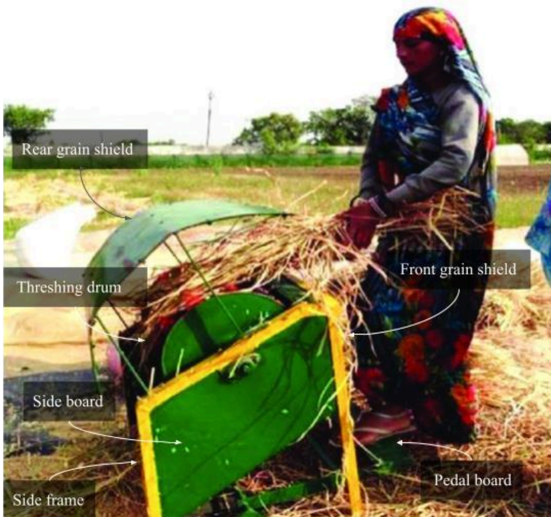
Figure 4.31: Manually operated pedal thresher. Adapted from Khadatkar et al. (2008)
