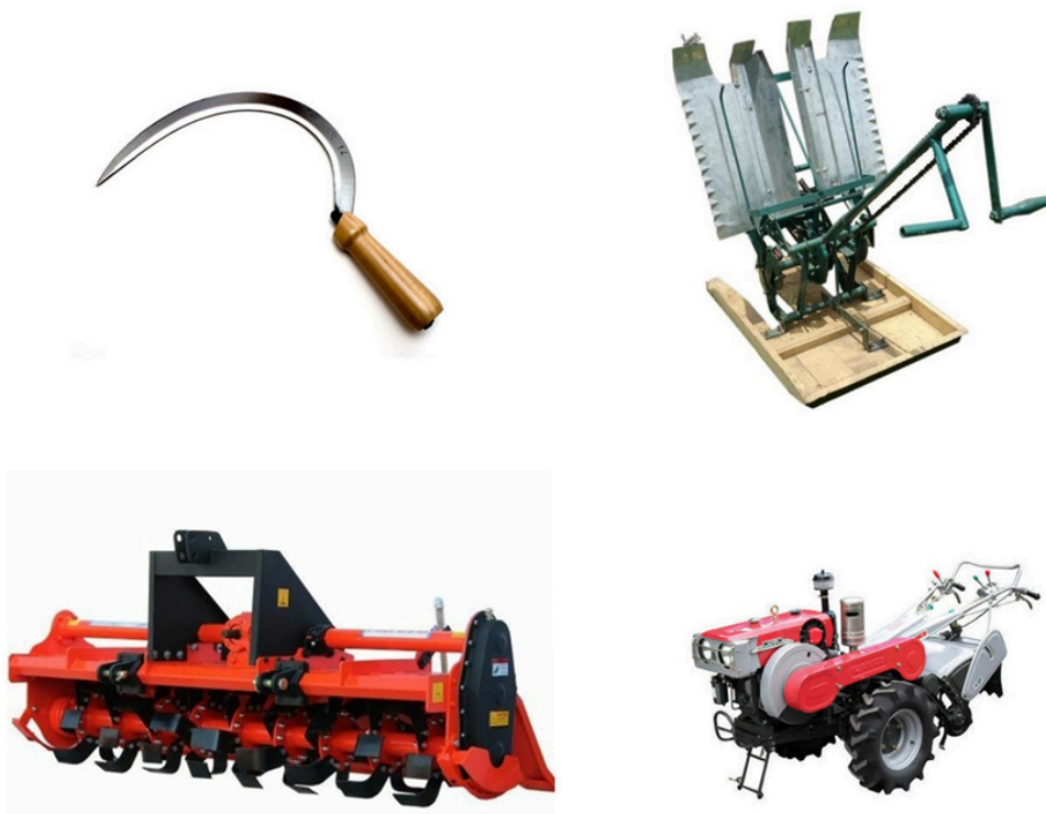
Figure 4.27: Examples of possible directions in tool design. Clockwise from top left, simple manual tool (sickle), complex manual tool (Rice transplanter), simple motor-driven equipment (power tiller) and complex tractor attachment (rotovator)
