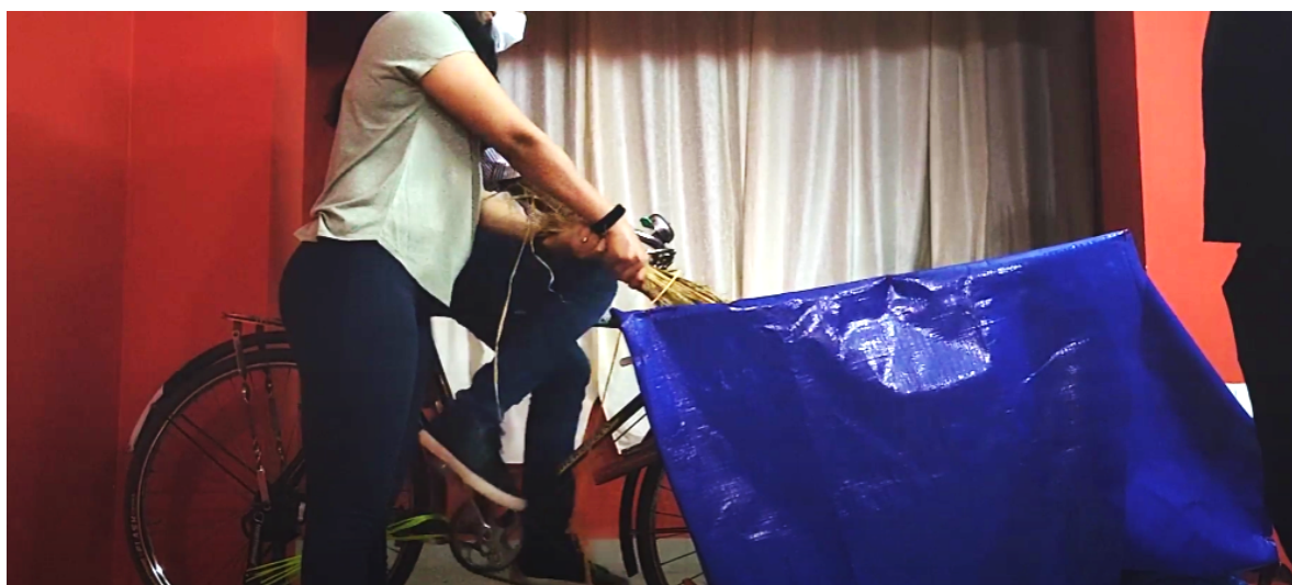
Figure 6.5: In-house test for threshing bundles of harvested rice panicles
