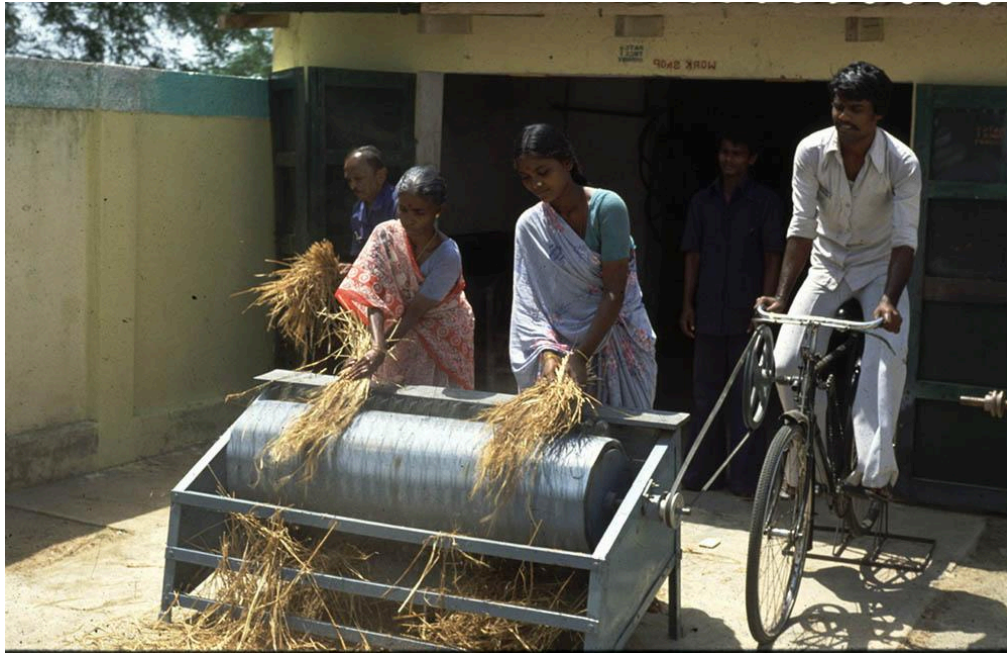
Figure 2.6: Dual Purpose Bicycle connected to a rice threshing device
