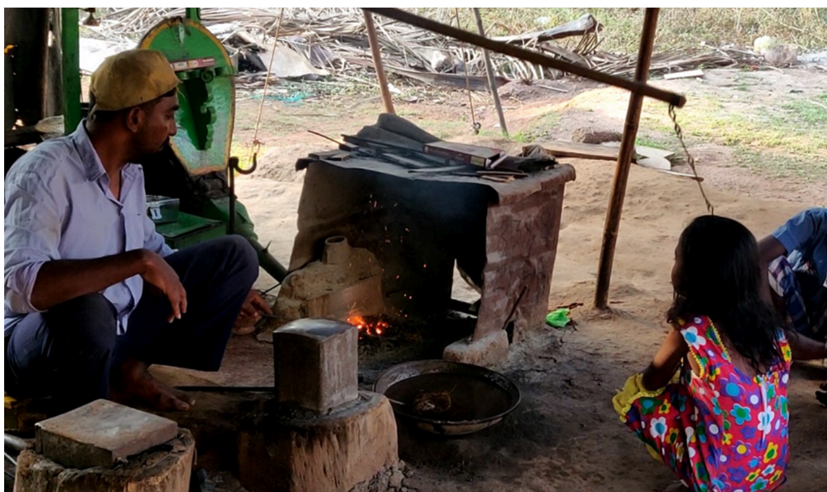
Figure 5.41: The village blacksmith using forging to repair a farm tool
