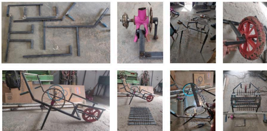
Figure 6.2: The stages of manufacturing the thresher prototype 2.0
