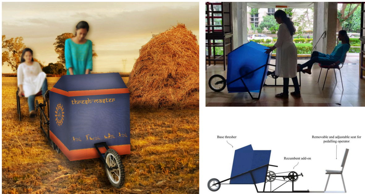
Figure 7.3: First design direction and prototype of a locally manufacturable thresher
