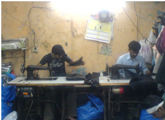
Fig.3.2(h) Assembly of all the parts: by stitching th bag inside out, to hide the seam line.
