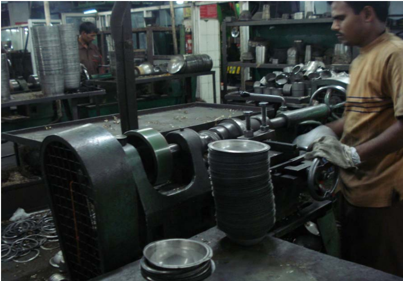
Shearing machine – cutting off edges
