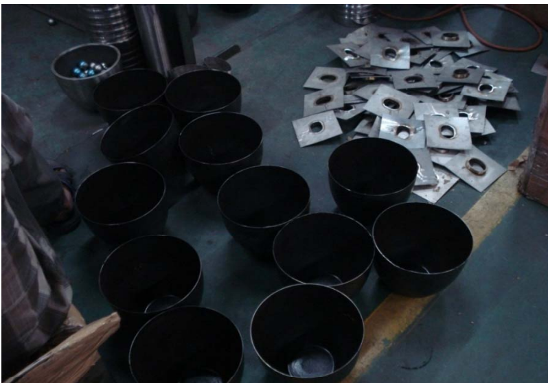
Single walled – before welding
