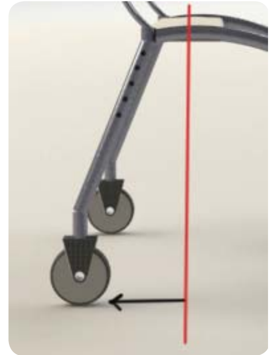
The front legs shall have to be moved outside to prevent the aid from toppling over when some one sits on it
