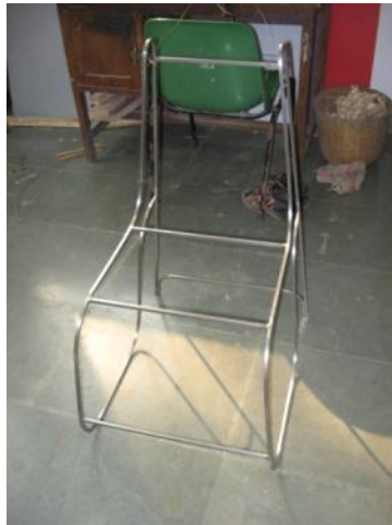
Wrought iron skeleton after polishing
