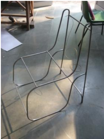
Wrought iron skeleton after polishing
