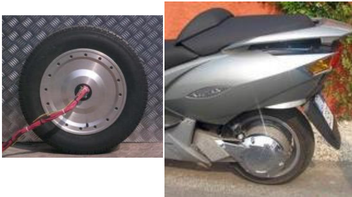
20kW hub mounted BLDC motor
