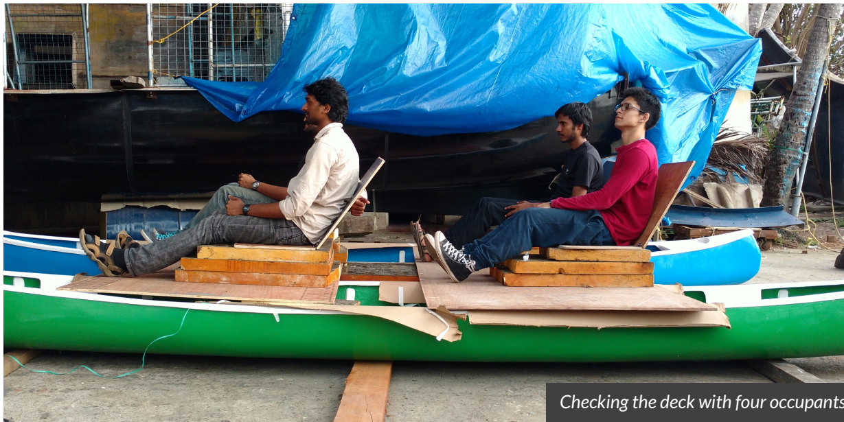
Mock up for finding the dimensions of the deck
