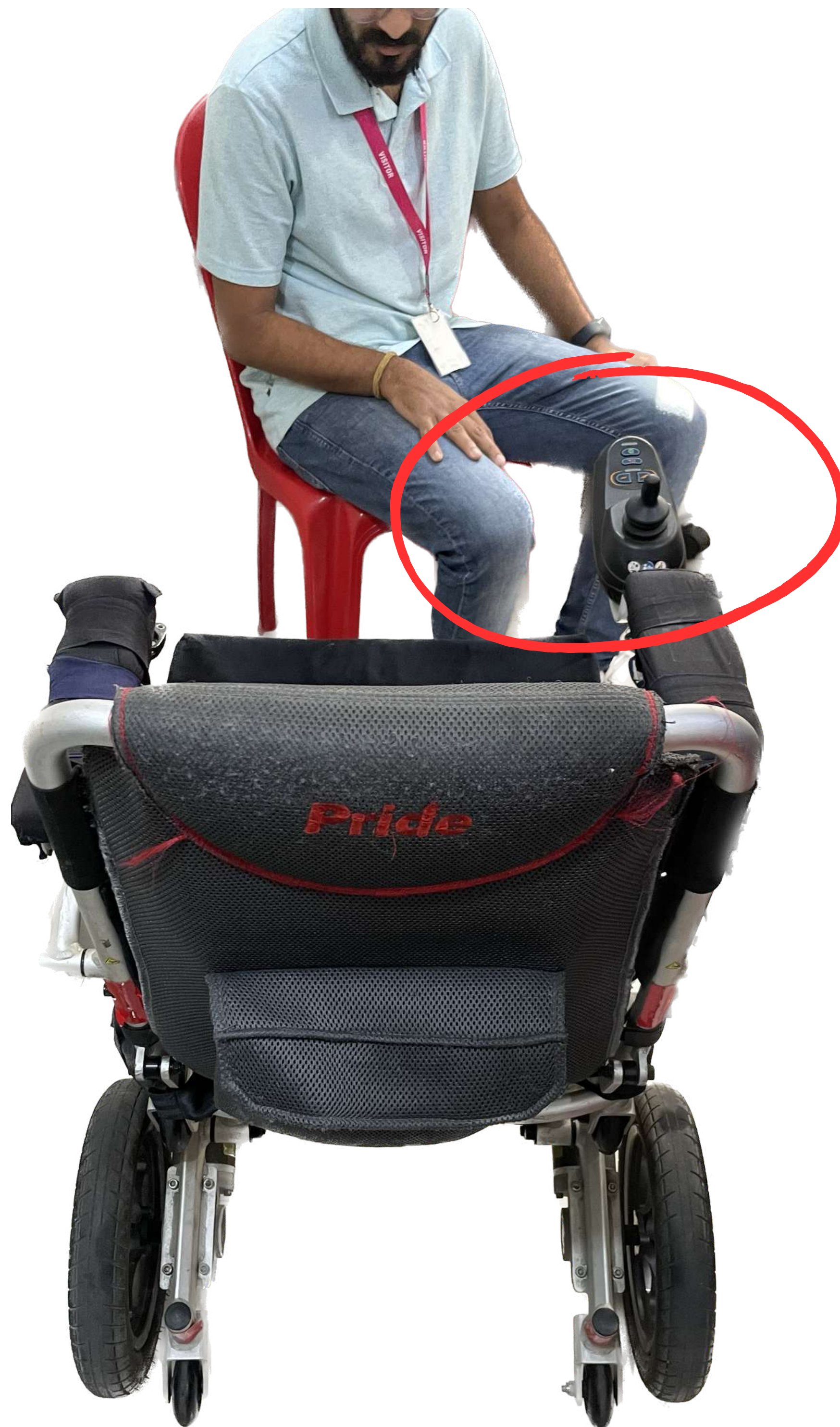
On the control handle, there is no adequate palm rest for the user
