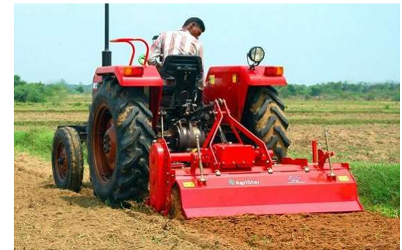
Rotavator used on dry land to pulverise the soil Pic 8
