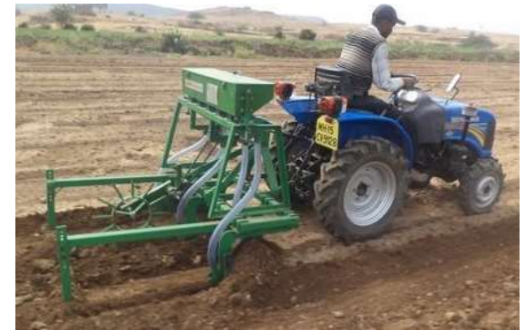
Seed drill implement used to sow grains Pic 10
