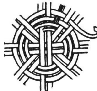
Round splint base with spokes in pair
