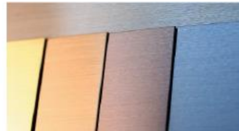
Stainless steel with Titanium coating
